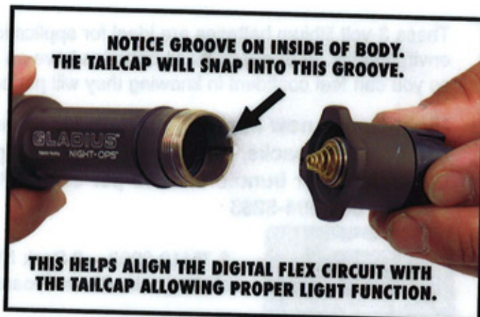
4. ALIGN TAILCAP AND BODY
